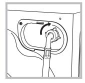
2. Connect the other end of the water inlet hose to the washing machine,
